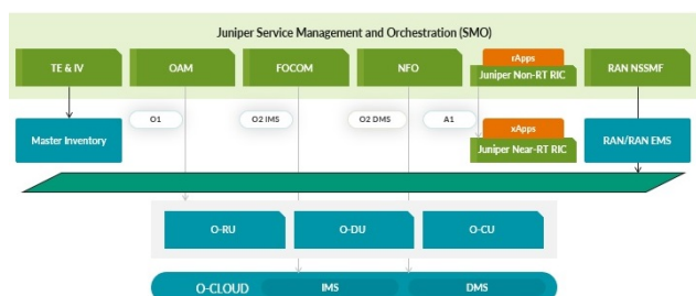
Figure 3: Juniper SMO is based on a cloud-native microservices architecture fully aligned to industry standards such as 3GPP, O-RAN, and TM Forum.
