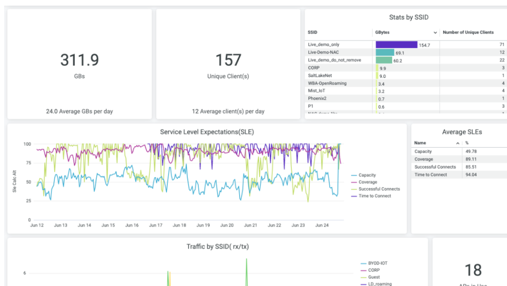
Figure 1: Top-level view of the Wireless Network Insights dashboard that includes organization-wide SLE and traffic trends; client distribution by device type, operating system, and 802.11 protocols; traffic and applications insights by SSID and clients; and more
